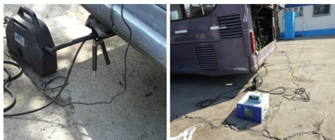
Fig.1. Analyzer set-up and the tailpipe emission testing operation.
